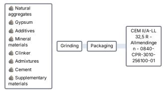
Cement is the key ingredient in concrete. When mixed with water and aggregates such as sand and gravel, it forms a paste that binds the aggregates together to create concrete, the most widely used construction material in the world.
