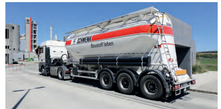
Cement silo semitrailer at the Mergelstetten plant | SCHWENK
