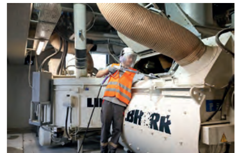
Cleaning the mixer in the ready-mix plant | SCHWENK
