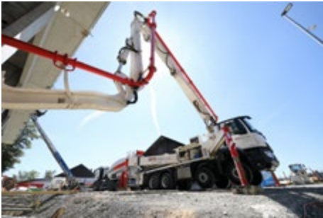
Picture: Concrete pump with secure stand, BPD Vogtland | SCHWENK
