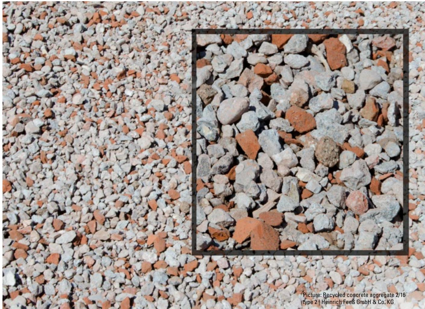
Picture: Recycled concrete aggregate 2/16 type 2 | Heinrich Feeß GmbH & Co. KG
